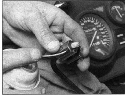
16.3a Lubricating a cable with a pressure lubricator. Make sure the tool seals around the inner cable
